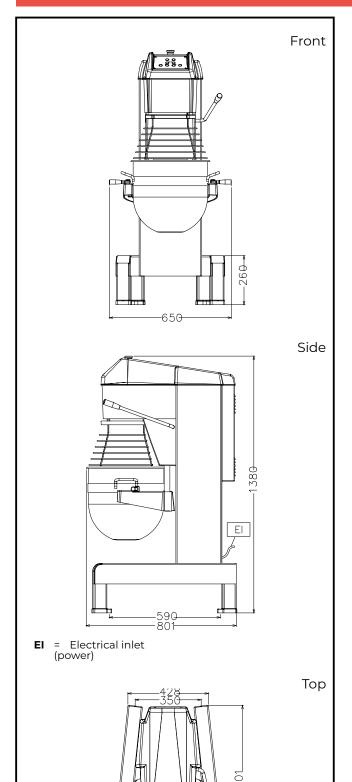
Electric Supply voltage: 200-240 V/1N ph/50/60 Hz Electrical power, max: 2.2 kW **Total Watts:** 2.2 kW Capacity: ISO 9001; ISO 14001 kg/ Performance (up to): Cycle 40 litres Capacity: Key Information: External dimensions, 655 mm Width: External dimensions, Depth: 850 mm External dimensions, 1370 mm Height: **Shipping weight:** 195 kg ISO 9001; ISO 14001 kg **Cold water paste:** with Spiral hook Egg whites: 70 with Whisk
